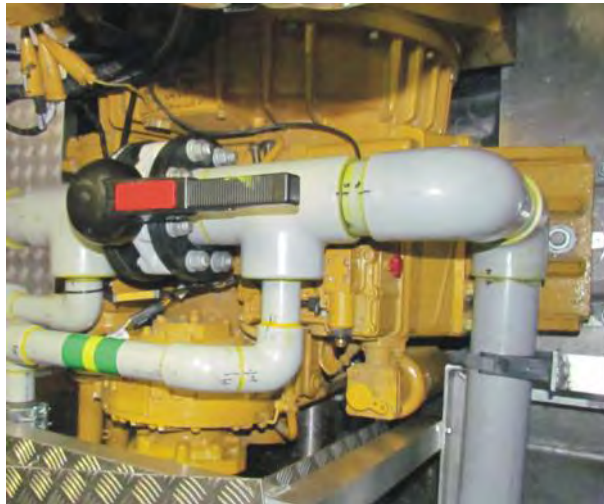
Figure 5-14: Gearbox Heat Exchanger and Flow Balance Valve
