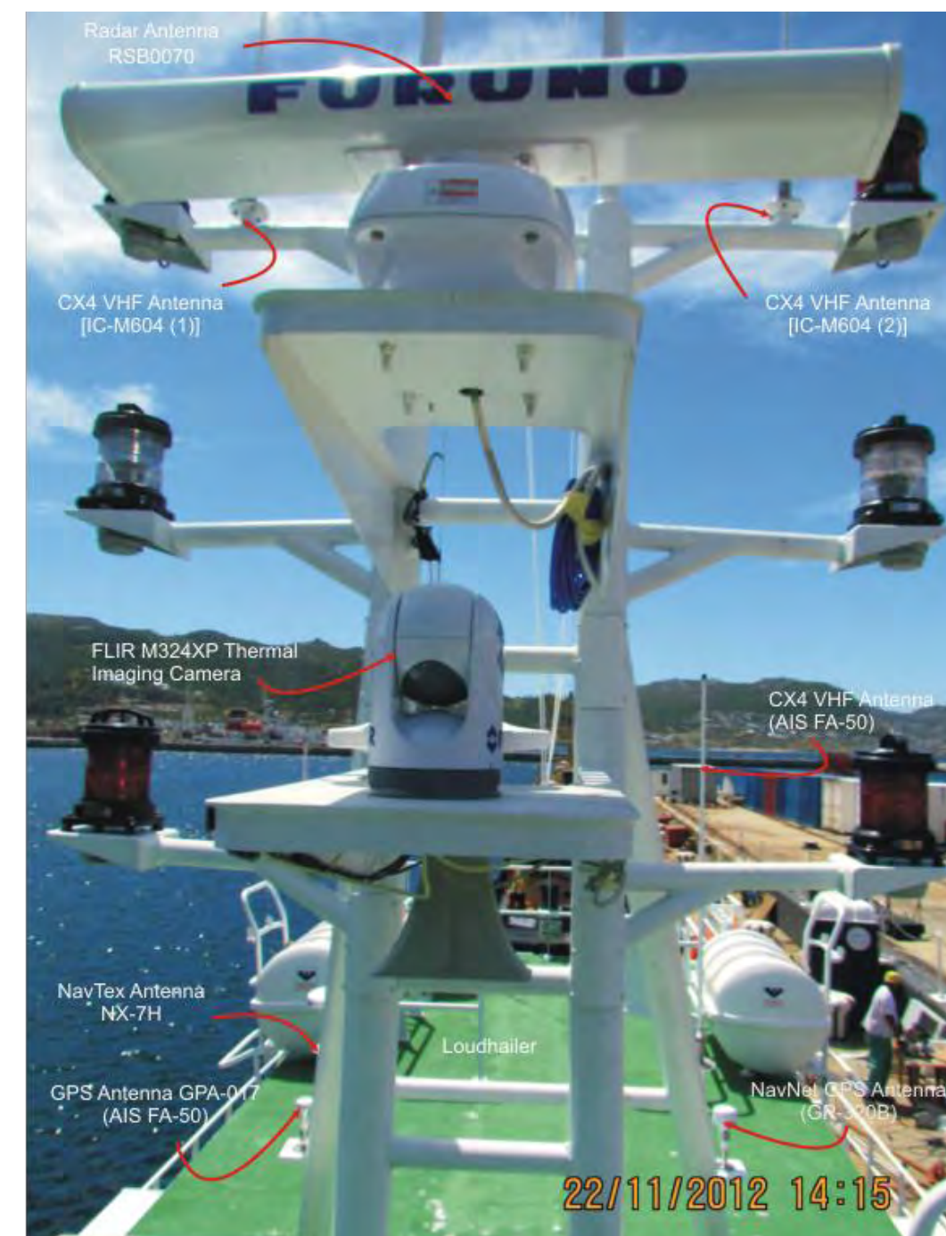
Figure 4-8: Mast Arrangement Identifying Antennae, Scanners, etc
